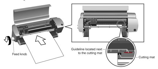
If the top edge of the sheet curls up and catches on the Craft ROBO, turn the feed knob in the direction toward the rear of the Craft ROBO to align the top edge of the sheet with the indented guidelines located behind the cutting mat. Please note, however, that the cutting area will be reduced by 5 mm in the media feed direction.
