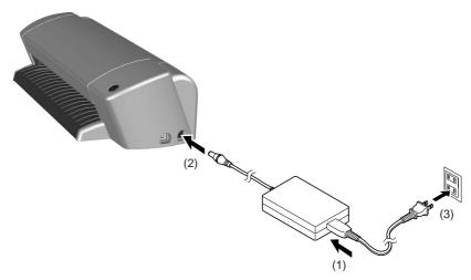
(4) Press the standby switch to turn on the power.
