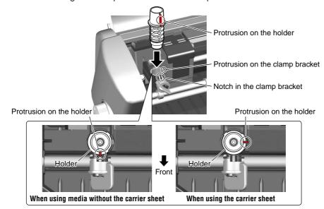
(2) Firmly insert the blade holder in the clamp bracket and then turn the lock lever to the right (CLOSE direction) to tighten the clamp bracket.
