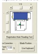
(5) Click the [Registration Mark Reading Test] button. After the Craft ROBO has read the printed cross, it will use the mounted blade to draw a cross.
