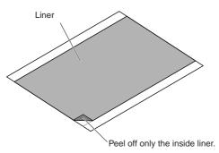
(2) Press the media onto the adhesive surface of the carrier sheet.
