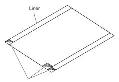
Peel off the inside liner and the liner strips on both sides of the carrier sheet.
